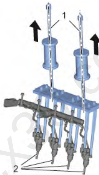
Fig. 98: Removing Fuel Injector Rail Assembly
